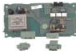
RS-485 Communications module (Includes EASYCOMM Software ) (for 14d and 14df computer only) R18011
