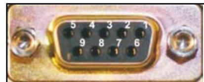
The DB-9 connector has the following configuration:
